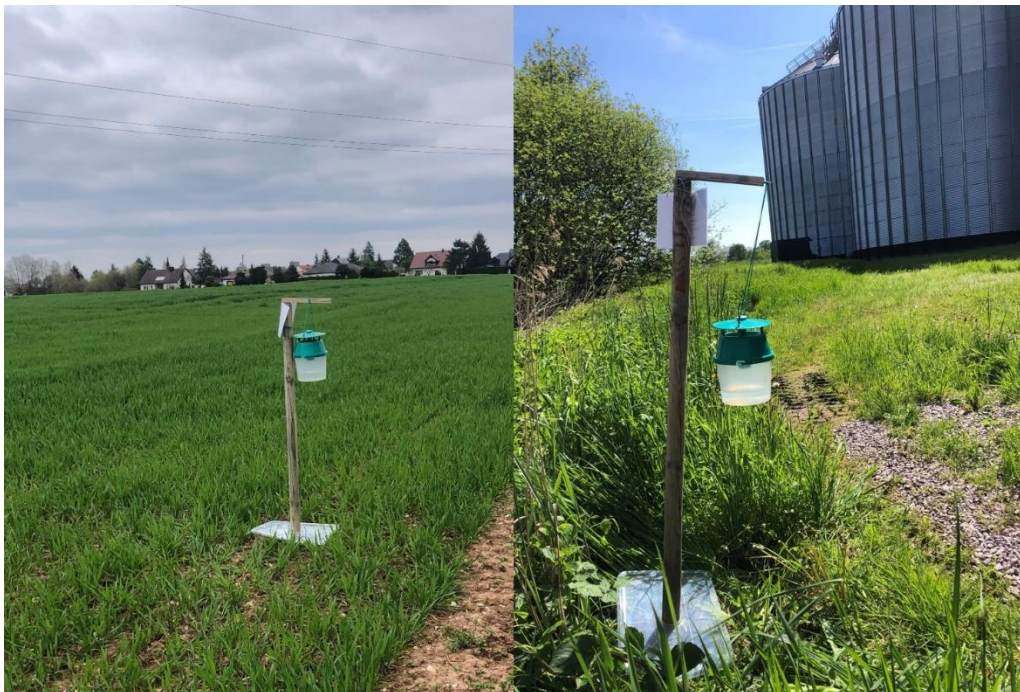
Figure 37 Traps for flying and crawling insects in the field (photo: C. Albrecht)
