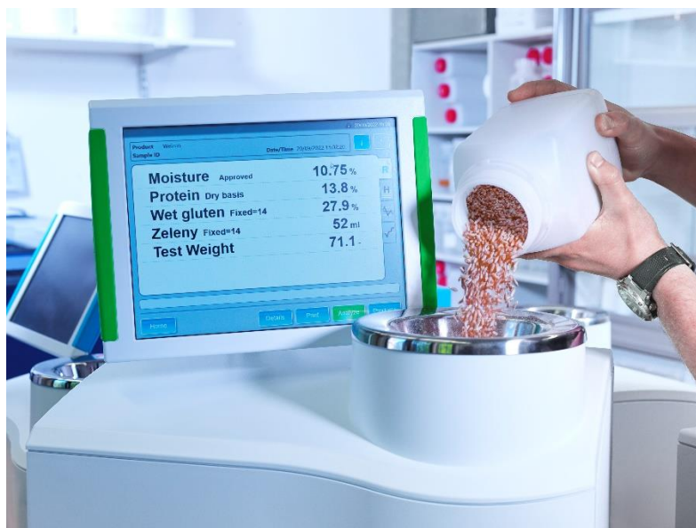
Figure 31 Measurement of moisture content (credit: PTB).
