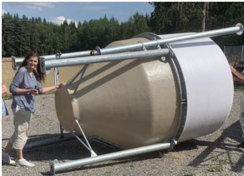
Figure 35 Hermetic glass fiber silo bin for above-ground storage tests (volume 6 m 3 , photo: C. Adler)
